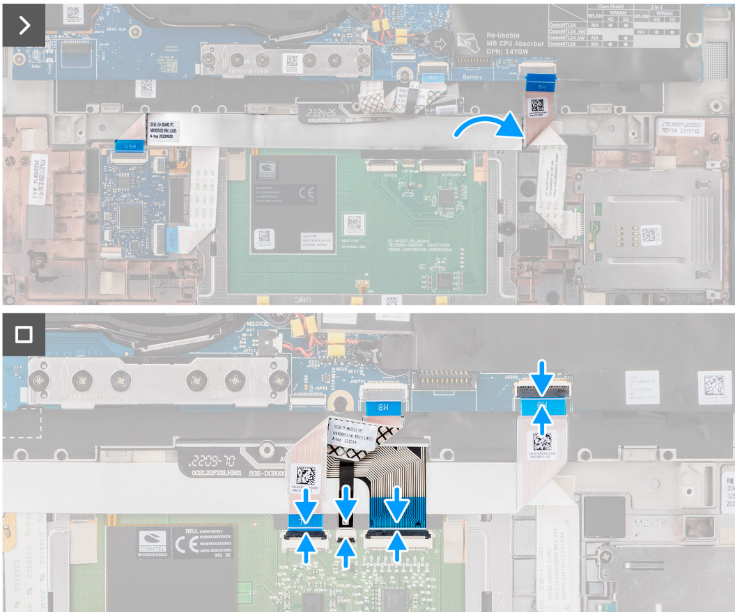
Figure 45. Installing the smart card reader
